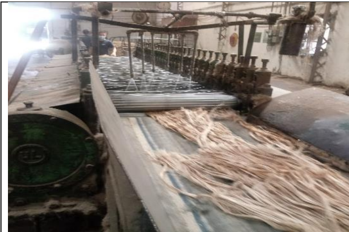
During process of the treatment of the fiber with emulsion blending at Agave Manufacturing mill on March 16, 2022
